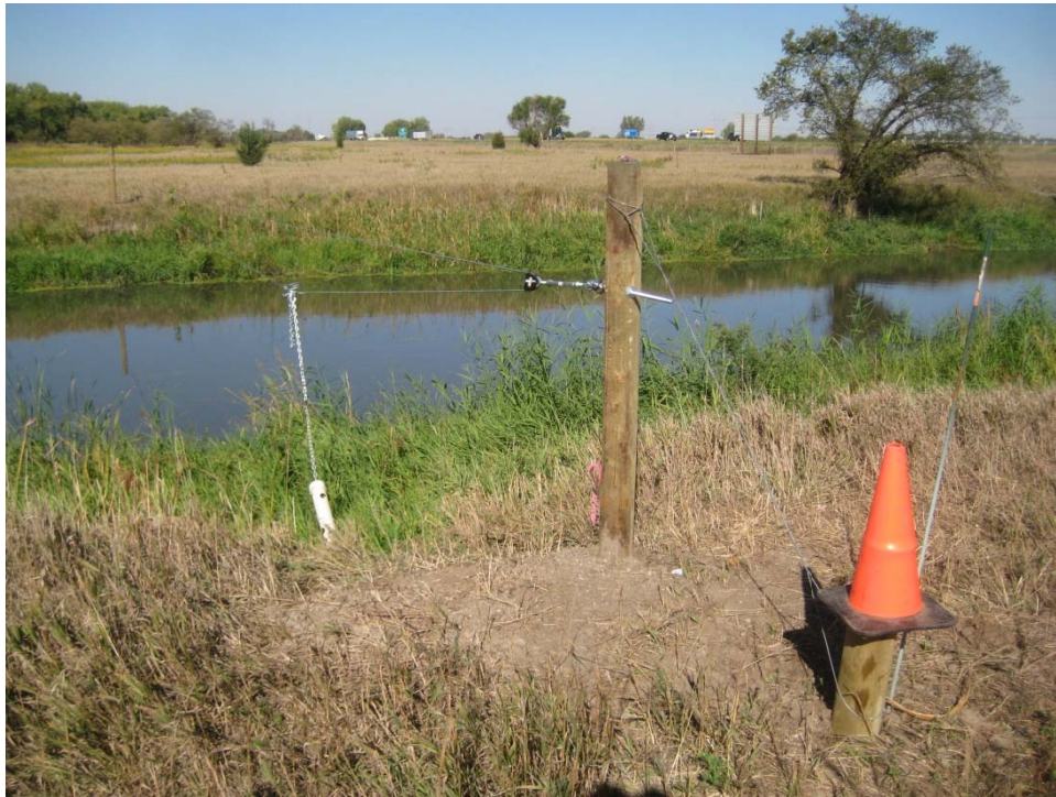
3. Manta 2 sonde deployment at Elm Creek near the confluence with the Platte River.
