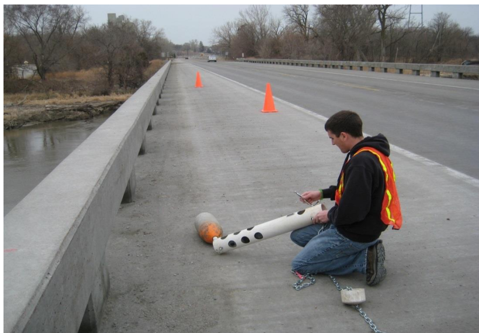
2. Manta 2 deployment on Hwy 50 bridge near Louisville, NE.
