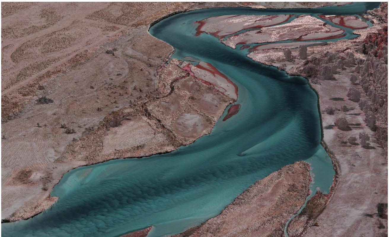
Figure 5: A view of the Platte River topobathymetric digital elevation model colored by elevation, and overlaid with the above-ground lidar returns colored using RGB imagery.
